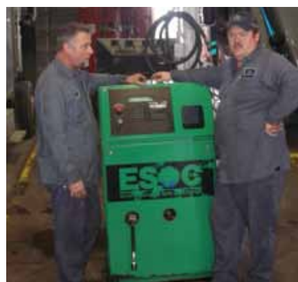
The fleet's ESOC Series 1000 engine oil exchange machine in positioned between two shop bays to enable technicians to do more oil changes without having to move trucks in and out as much, increasing technician and shop productivity. Technicians Bruce Kuka, left, and Brian Mattson, right, say the machine cuts down on the time and effort needed to change oil, with less mess for a cleaner work environment.
